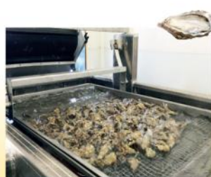
Vibrating grader for oysters Up to 5 grades
